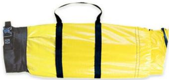
The VB1 Air Duct Blower hose is available with a convenient self-storage and carry Store Sak for 25 foot lengths. Single-ply PVC vinyl coated polyester fabric reinforced with a spring steel wire helix & external PVC wearstrip. Same Quality VB1 Hose, but Easily Transported. For temporary air flow. 6" to 24" diameters. -20F to 180F.
